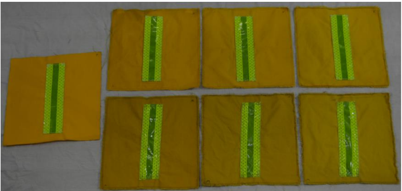
3 INCH PERFORATED DIAMOND TRIPLE TRIM LAUNDERED SWATCHES TOP: XEROS OUTERSHELL LAUNDERING 10 CYCLES, 30 CYCLES, 50 CYCLES BOTTOM: MILNOR OUTERSHELL LAUNDERING 10 CYCLES, 30 CYCLES, 50 CYCLES LEFT: PRISTINE
