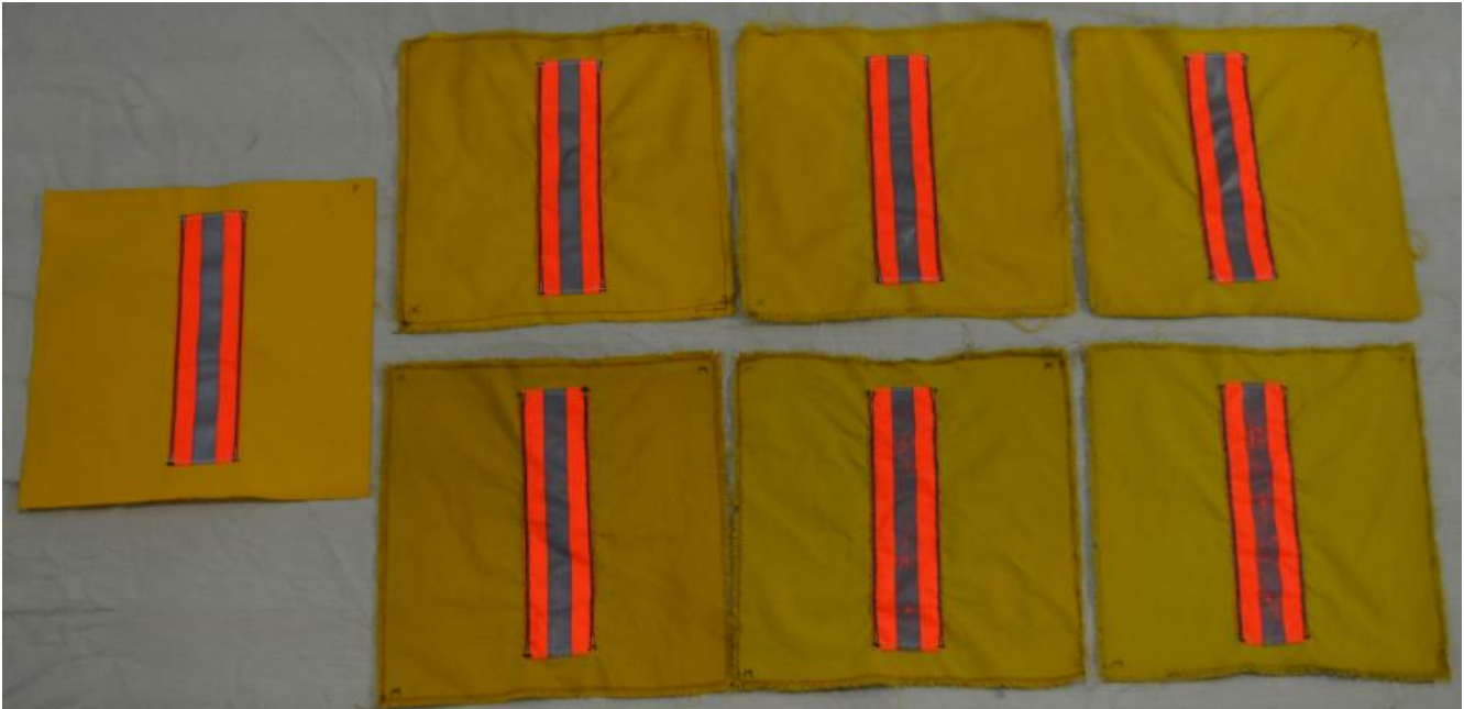
3 INCH TRIPLE TRIM ORANGE WITH TRIM TRAX LAUNDERED SWATCHES TOP: XEROS OUTERSHELL LAUNDERING 10 CYCLES, 30 CYCLES, 50 CYCLES BOTTOM: MILNOR OUTERSHELL LAUNDERING 10 CYCLES, 30 CYCLES, 50 CYCLES LEFT: PRISTINE
